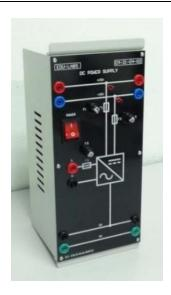
Output Type: DC Fixed Output Voltage
