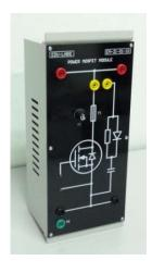
: Power Field Effect Device Transistor (N-Channel Enhancement Mode Silicon Gate)
