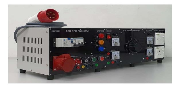
The system designed to provide all fixed and variable AC and DC supplies which necessary in an electrical machines laboratory to perform the experiment required and work project.
