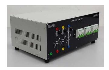
Single & Three phase Capacitive Load 7 steps variable per phase
