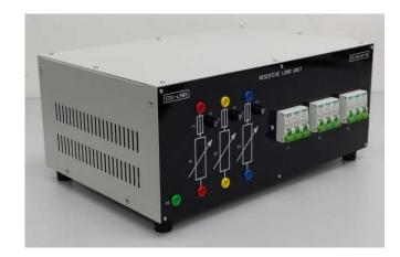
Single & Three phase Resistive Load 7 steps variable per phase
