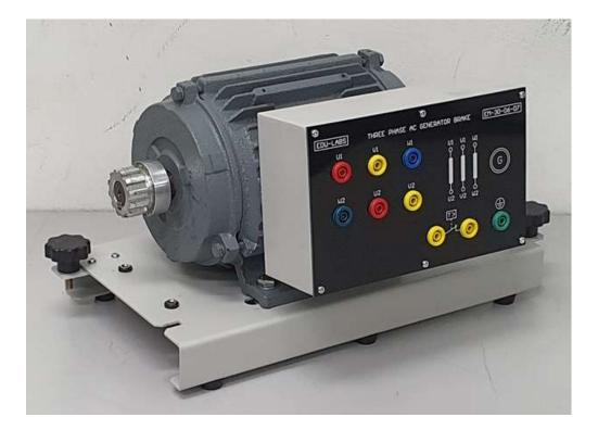
AC three Phase generator type for testing mechanical load characteristics, convenience to measuring output torque & speed of motor on testing by attach to Prime Mover, Torque Sensor & Controller. To measure the characteristics of torque and speed.
