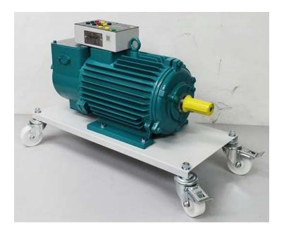
Three Phase slip ring induction motors, the rotor is actually "wound on an armature". The windings are brought out to terminals by a set of three "slip rings" on the armature shaft. Three phase winding both stator and rotor induction motor with slip ring at the rotor end. Winding terminals of K, L & M brought out for external Rotor Resistance Starter application.
