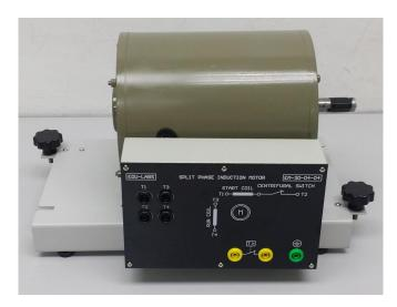
Single phase asynchronous induction motor with split phase construction.
