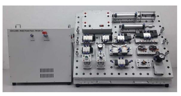
The FW-202 is consists of actual industrial grade modified aluminum pneumatics parts which are commonly apply and used in industrial field. It is classified into basic level, intermediate level and up to advance level training experiments.
