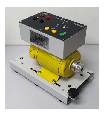
DC Motor / Generator Operation, suitable for shunt excited connection
