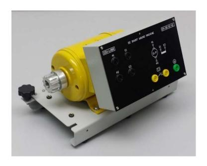
DC Motor / Generator Operation, suitable for series excited connection
