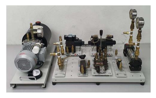
The Basic Hydraulics Trainers FH-201 is consists of actual industrial grade hydraulics components and parts which are commonly apply and used in industrial field. It is classified into basic level training experiments.
